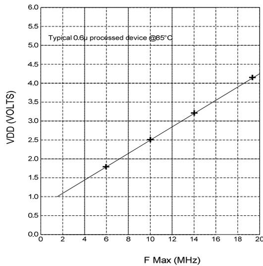
Figure 4-2b W65C22S F Max vs. VDD
