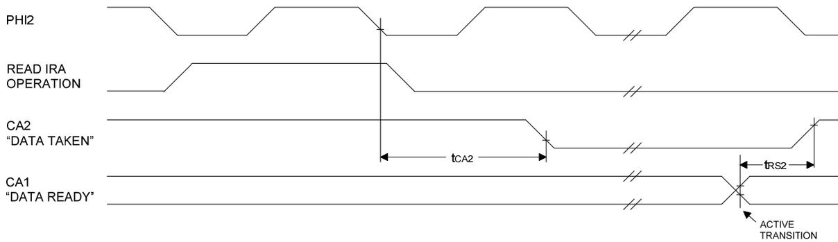
Figure 4-4 Read Handshake, Handshake Mode Timing (CA2)
