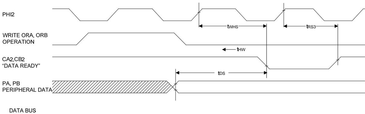
Figure 4-5 Write Handshake, Pulse Mode Timing (CA2, CB2)
