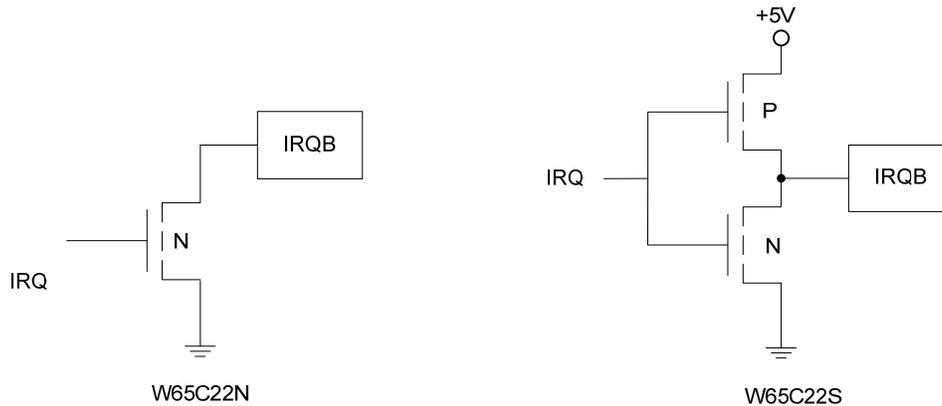
Figure 3-4 IRQB Buffer - W65C22N and W65C22S
