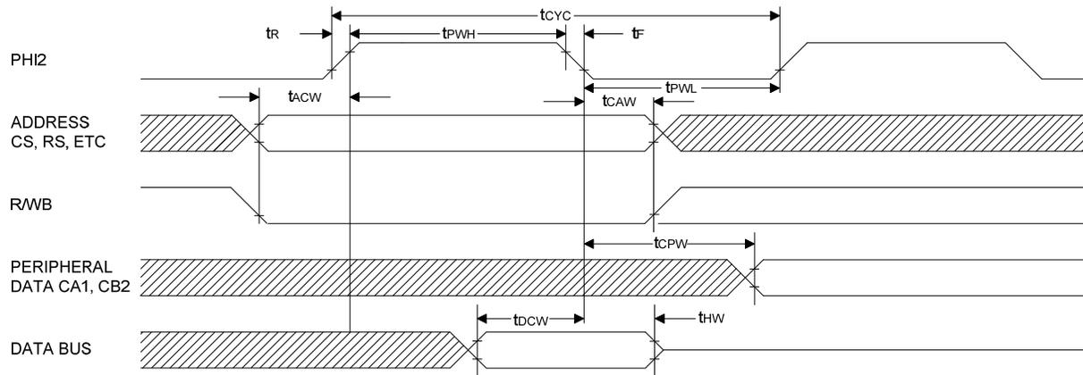
Figure 4-2 Write Timing
