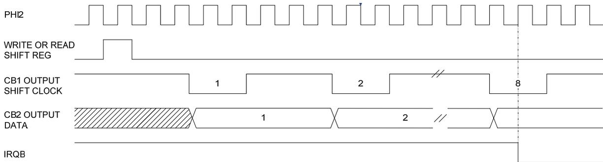
Figure 2-12 Shift Out - External CB1 Clock Control Timing
