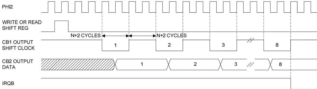
Figure 2-10 Shift Out - T2 Control Timing
