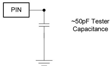
Figure 4-12 Test Load (All Dynamic Parameters)
