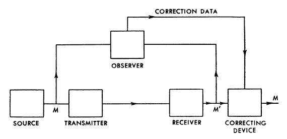
Fig. 8. — Schematic diagram of a correction system.
