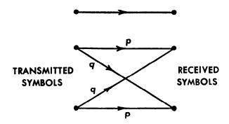
Fig. 11. — Example of a discrete channel.
