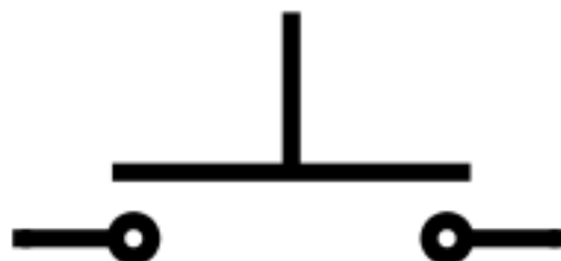
Figure 9: The switch symbol comes in many forms. This is the pushbutton switch.
