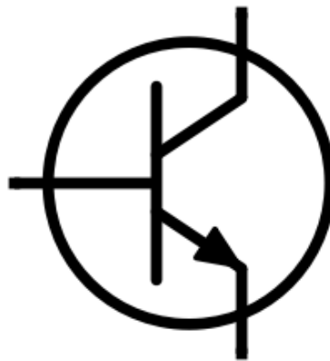
Figure 16: The transistor symbol for a NPN transistor
