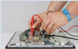
FIGURE 12.3.2 When building, testing or repairing electronic circuits, technicians use a wrist strap to ground their body, to ensure no static electricity is transferred to the electronic circuit.
