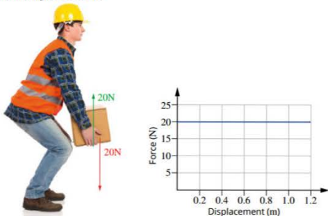
FIGURE 5.2.6 The force–displacement graph for this person lifting a box is a straight, horizontal line, indicating that the force applied to the box is constant throughout the process.
