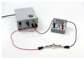
FIGURE 13.1.7 A digital ammeter (labelled with an A) measures current in a circuit.
