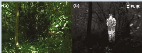
FIGURE 11.6.4 (a) The person standing behind the bush is difficult to see in normal light, but (b) they are warmer than the vegetation surrounding them and produce a stronger infrared emission, which a thermal imaging device is able to detect.
