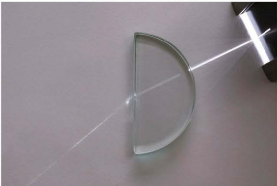
FIGURE 10.2.1 Light refracts as it moves from one medium (i.e. the semicircular glass prism) into another (i.e. air) causing a change in direction.
