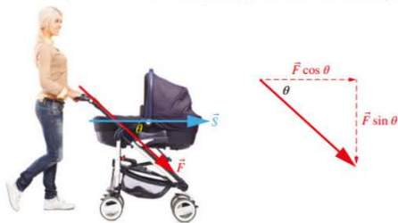
FIGURE 5.2.5 When a person pushes a pram, the force applied by the person can be resolved into a horizontal force and a vertical force.
