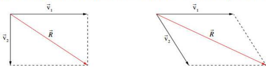
FIGURE 3.1.6 Parallelogram of vectors method for adding two vectors.
