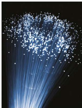
FIGURE 10.2.5 Optical fibres transmit light using total internal reflection.
