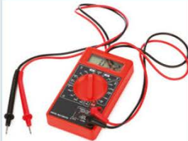
FIGURE 13.2.8 A digital multimeter can be used as either an ammeter or a voltmeter.
