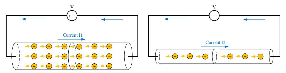
Even with the same voltage, the resultant currents in the two cases are different. The wire with larger diameter allows more charges to pass through the cross section at a time than that of the wire with smaller diameter, meaning that **I1 is larger than I2**.
