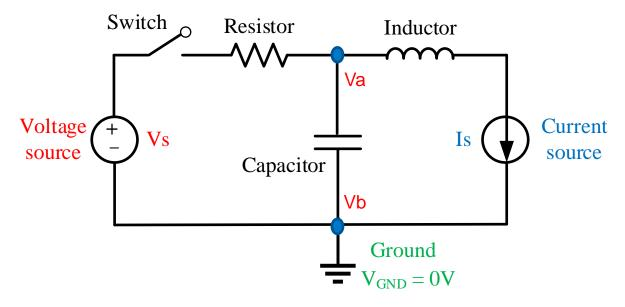
Voltage source provide constant voltage output but we don't know the current passing through it.
