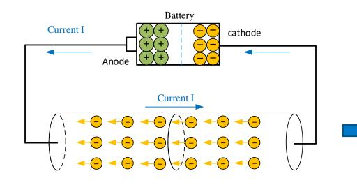
We usually label the node with higher potential with "+" and the node with lower potential with "-". The current flows from "+" to "-".
