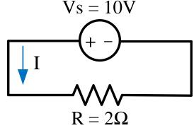
One can easily determine using Ohm's law that the current go through the resistor is I = V/R = 5 A.
