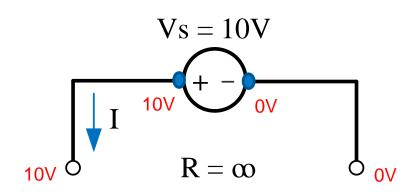
Follow the current direction, there is always a voltage drop. The value of voltage drop can be calculated using Ohm's law.
