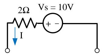
The voltage across the resistor is 0 because the current is 0.
