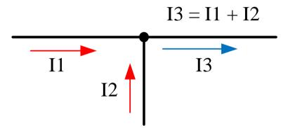
If we assign a mathematical sign (polarity) to each current, denoting whether they enter or exit a node, we can use the equation  $\Sigma I_{IN} = \Sigma I_{OUT}$  to find out the unknown current.
