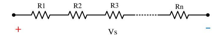
$$V_m = \frac{V_s R_m}{R_1 + R_2 + \dots R_n}$$
