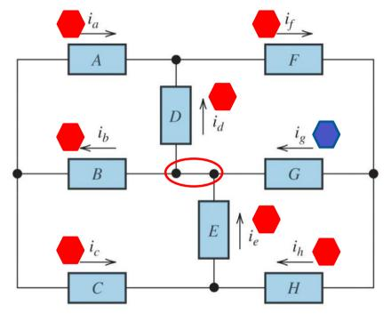
Two electrically common nodes can be seen as a super node:
