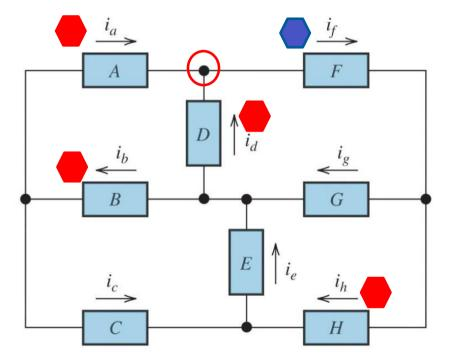
KCL:  $\Sigma I_{IN} = \Sigma I_{OUT}$
