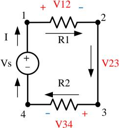
**Step 4:** Use Ohm's law to get the value of the voltage drops to complete the equation. In this case,  $V_{12} = IR1$ ,  $V_{34} = IR2$ .
