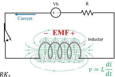
The solution of this kind of equation for the variable is always in the following format  $i = K_1 e^{st} + K_2$
