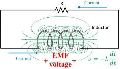
During the discharging process, we need to include the minus sign in the voltage generated by inductor.
