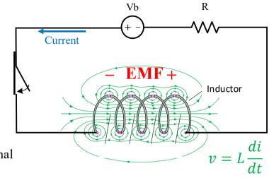
The solution of this kind of equation for the variable is alwavs in the following format  $i = K_1 e^{st} + K_2$
