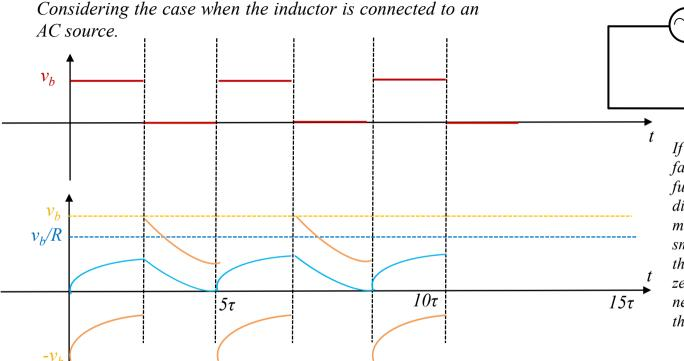
If the voltage source changes fast, before the inductor got fully charged, it already started discharging. Therefore, the maximum current it can have is smaller than the DC case. And the voltage will never reduce to zero. The source will always need to split some voltage on the inductor.
