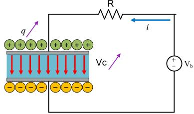
At  $t = \tau$ , the current was reduced to 37% of the maximum value and the voltage was increased to 63% of the maximum value.
