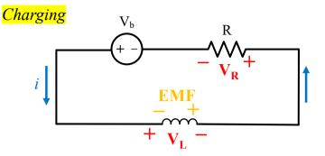
The EMF voltage generated by the inductor is negative, the source needs to split a part of its voltage to overcome this EMF.
