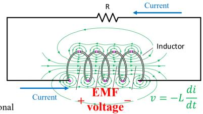
The solution of this kind of equation for the variable is always in the following format  $i = K_1 e^{st} + K_2$
