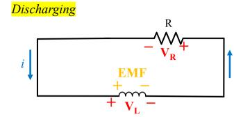
The EMF voltage generated by the inductor is positive as the current is decreasing and it serves as the source of the circuit.
