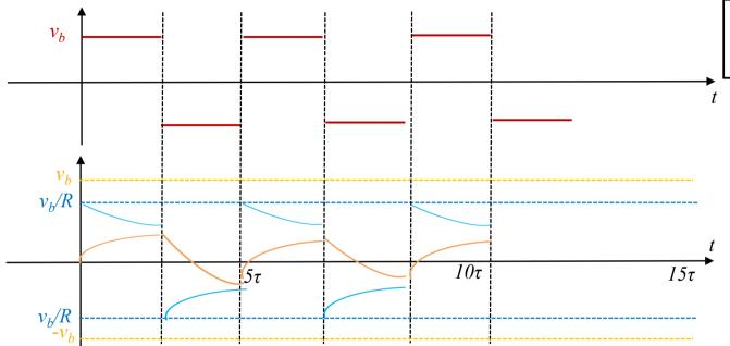
$v_R$  C  $V_C$ If the voltage source changes fast, before the capacitor got fully charged, it already started discharging and charging in the other direction. Therefore, the
