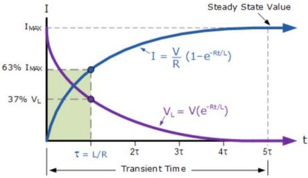
At  $t = \tau$ , the current was reached to 63% of the maximum value and the voltage was reduced to 37% of the maximum value.
