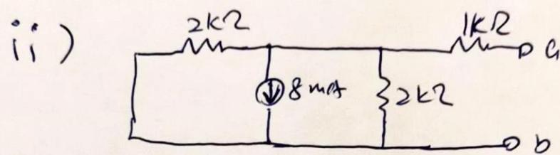
$$V_{ab-2} = -8 \times \frac{1}{2+1} = -8V$$
