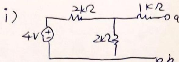
$$V_{ab-1} = 4V \times \frac{2}{2+2} = 2V$$
